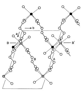
Fig. 2. Structure of calcium succinate trihydrate projected down the c\* axis. The filled circles represent Ca atoms at z=1/2 and the shaded circles the Ca atoms at z=0.
